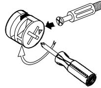
The head of the cam bolt goes into the open mouth of the cam nut. You then turn the cam nut so it tightens over the bolt.
