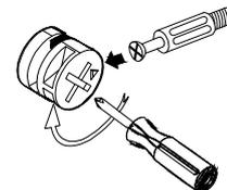
The head of the cam bolt goes into the open mouth of the cam nut. You then turn the cam nut so it tightens over the bolt.
