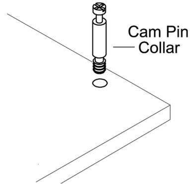
The Cam Pin is inserted into the flat side of a board, it is important that: The cam pin is kept vertical and is not put in on an angle.
