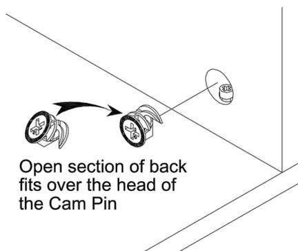
Insert the Cam Lock into the large hole so the opening of the "C" fits over the head of the Cam Pin. You must ensure that the Cam Lock is pushed to the bottom of the hole to catch the top of the Cam Pin.
